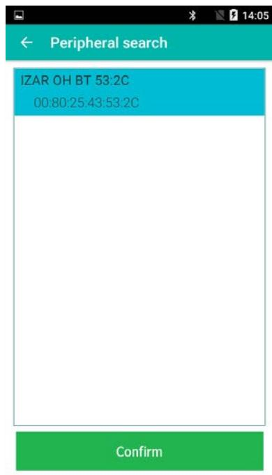
In this window, you can pair an optical head IZAR OH BT in order to perform a radio reading of the Diehl Metering products (PRIOS, REAL DATA and OMS protocols).
