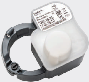
Diehl Metering has invested in improving the recyclability of its clip-on radio modules for water metering. Thanks to the solution, which is currently being rolled out, the electronics and battery will no longer be potted, making them easier to access and recycle.
