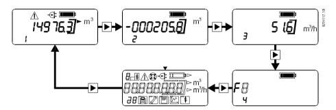
Figure 6-1 Operating the local display
