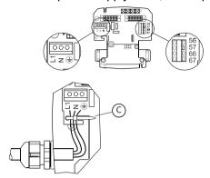
4. Tighten cable gland for power supply cable (approx. 20 Nm).
