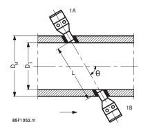
Figure 3-2 Measuring principle
