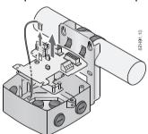
3. Smoothly push the cables one by one from underneath the base through the glands and adjust all cable ends approximately 100 mm from the upper frame of base.
