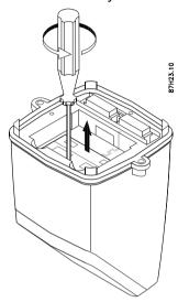
2. Fit new battery pack in transmitter.
