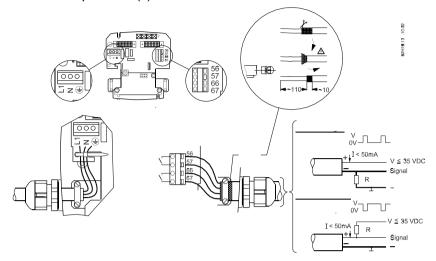
4. Tighten cable gland for output cable(s) (approx. 20 Nm).
