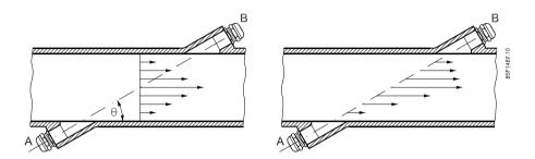
Figure 3-1 Velocity distribution along sound path
