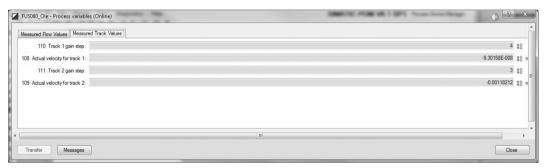
The **Measured Track Values** tab shows the gain steps and the flow velocities for path 1 and path 2. For 1-path applications the values for path 2 (track 2) are 0.
