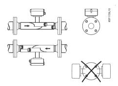
In horizontal installation avoid any upward/downward position of the transducers.
