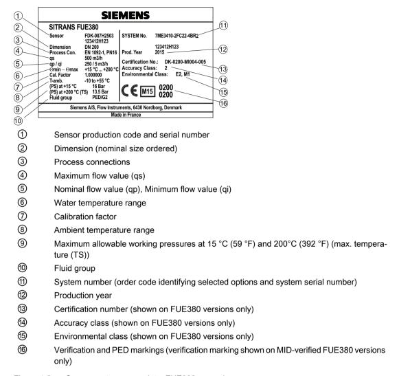
Figure 1-2 Sensor system nameplate, FUE380 example
