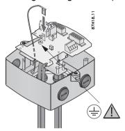
5. Tighten both transducer cable glands to ensure they are firmly sealed (recommended torque: approx. 20 Nm)
