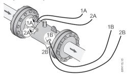
2. Snap out the connection plate and loosen the grounding wire.
