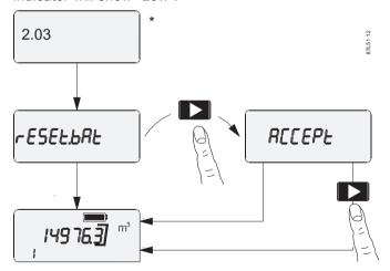
Figure 6-2 Reset internal battery counter
