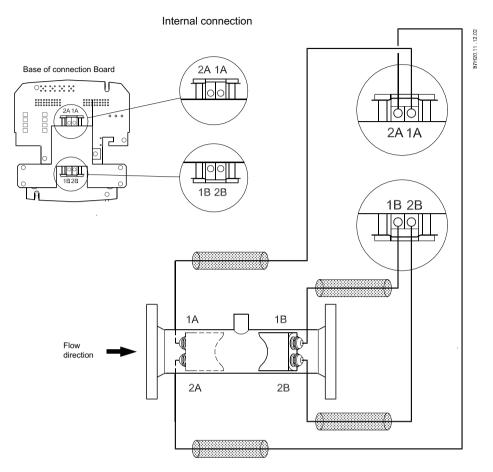
Figure 5-1 Wiring diagram, base of connection board
