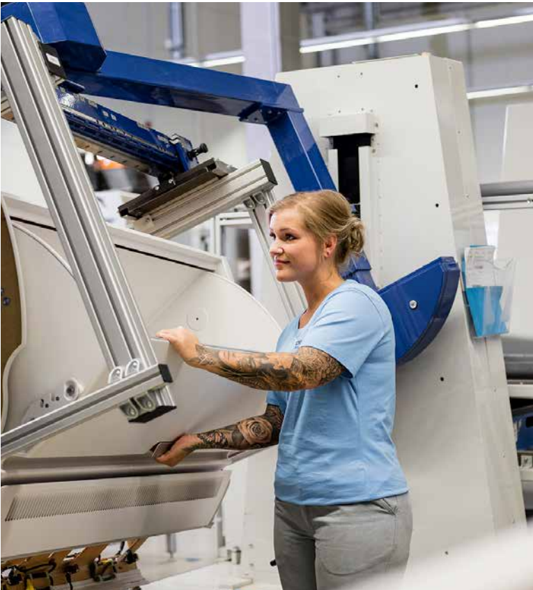
On the finishing straight: The final touches to the overhead bins – shortly before final assembly.
