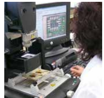
High-precision fitting and soldering of opto-electronic components
