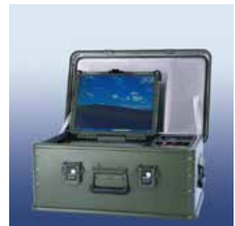
Fire Command Unit – for easy integration of new ammunitions into existing weapon systems.
