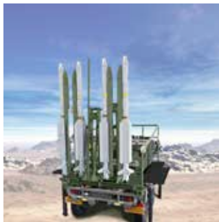
Launcher for IRIS-T SLS (surface-launched short-range) missiles
