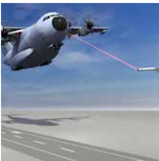
Laser systems protect transport aircraft against missile attacks
