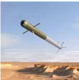
The 70 mm GILA guided missile is offered for the Tiger helicopter for precision fire support of ground troops.
