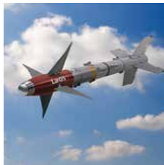
Laser-Guided Sidewinder – air-to-ground guided missile with semi-active laser for engaging land targets from various carrier platforms.
