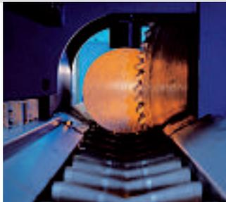
Cutting the bars / block saw
