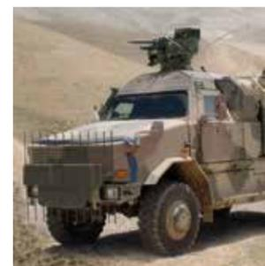
Counter-IED: Vehicle with front-mounted HPEM<sup>1</sup> effector system for protecting military convoys against IEDs.
