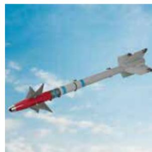
Laser-guided Sidewinder – air-to-ground guided missile with semi-active laser for engaging land targets for various carrier platforms.
