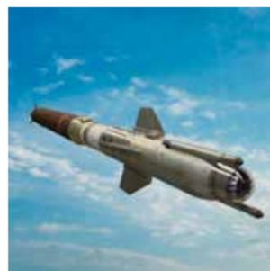
The RAM Block 2 guided missile features an upgraded radar seeker head and highly improved agility.
