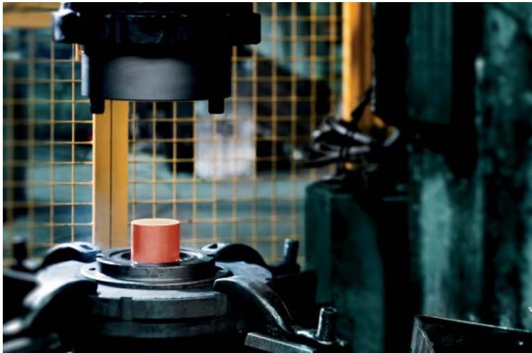
Bringing the billet to temperature and placing it in the die
