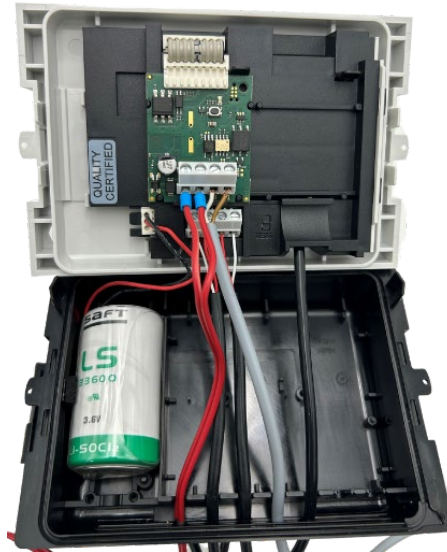
Figure 7 Connecting the EIA-485 interface
