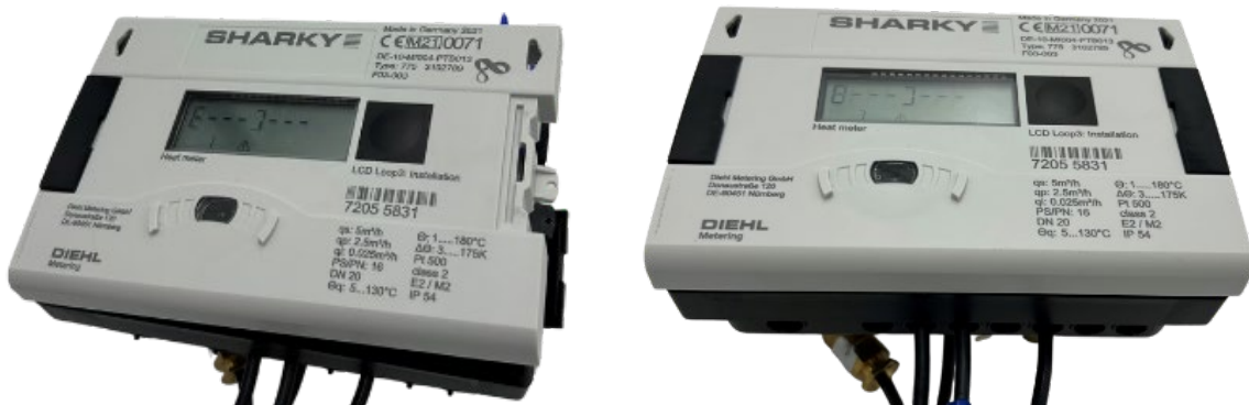
Figure 8 Closing the meter housing starting from left edge then closing the meter housing with the side latches
