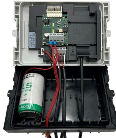
Figure 5 Example of power supply wiring
