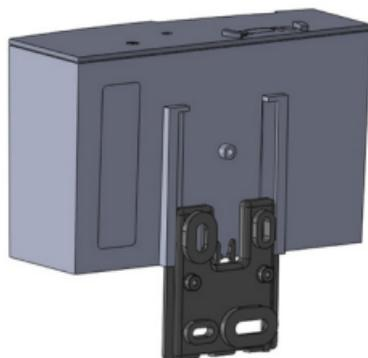
2. Push the module into the fixture plate from above until it engages in the locking pin.
