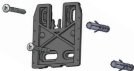
1. Use the two screws (and dowels) to properly attach the wall bracket to a wall.
