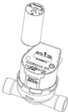
For correct configuration, the optical head must be placed on the optical interface.
